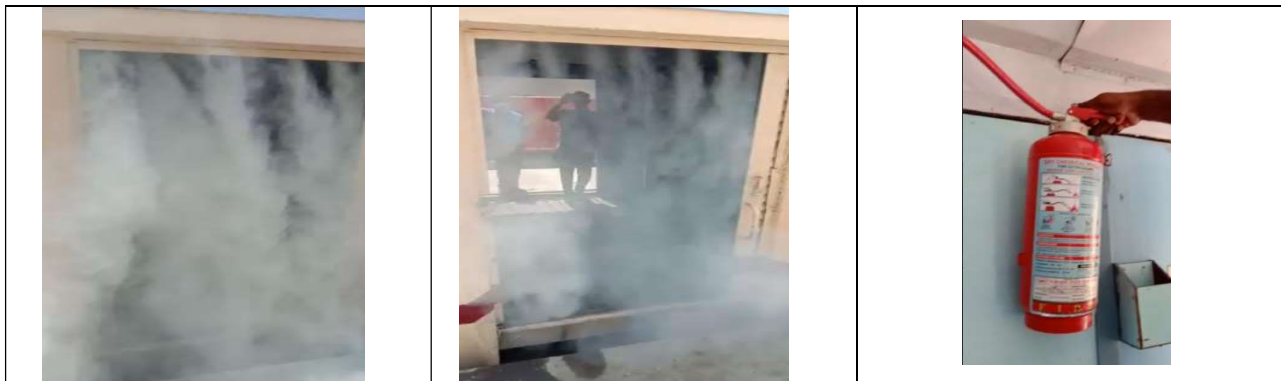
Remote operation of fire extinguisher cause spray of DCP in side luggage compartment
